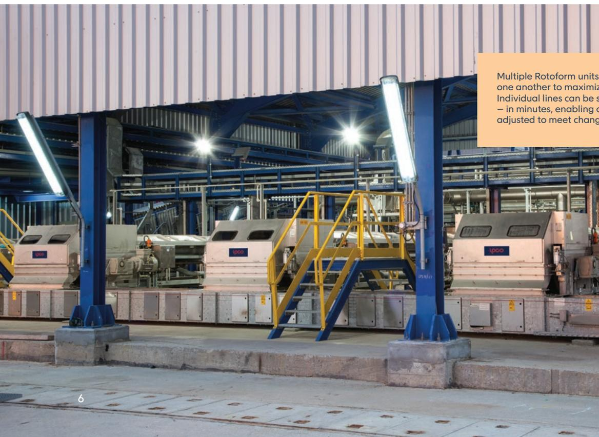
Multiple Rotoform units can be installed alongside one another to maximize production flexibility. Individual lines can be shut down – and restarted – in minutes, enabling overall capacity to be adjusted to meet changing throughput rates.
