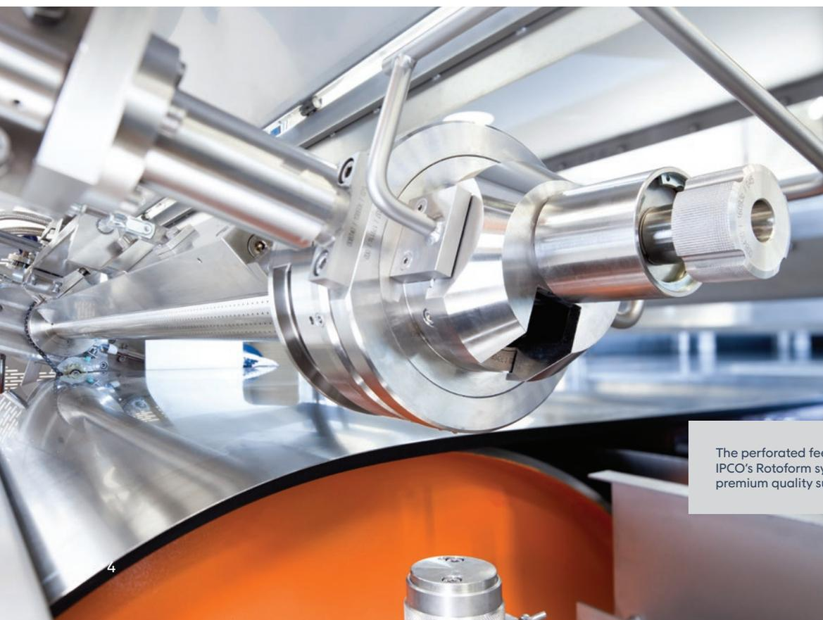
The perforated feed device on IPCO's Rotoform system helps ensure premium quality sulphur solidification
